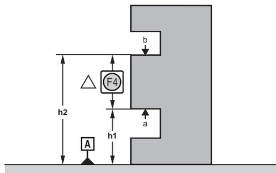
**MODE 2 Measuring length in two directions, with calibration**
