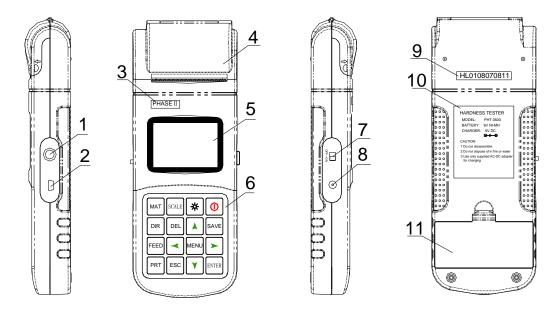
Socket of impact device 2 USB port 3 Phase II 4 Paper compartment cover
