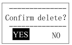
Press key [ ] or key [ ] to move the cursor to [YES] or [NO]. Press key [ ENTER ] to confirm operation. Press key [ESC] to cancel delete operation.
