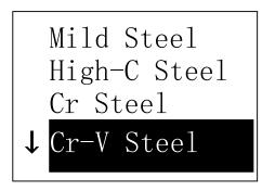
Press key 【▲】 or 【♥】 to move the cursor to the material to want to preset. Press key 【ENTER】 to confirm it. Press key 【ESC】 to cancel it.
