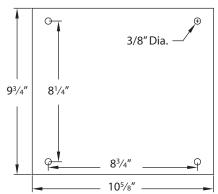
Figure 2 – Base Dimension and Mounting Holes
