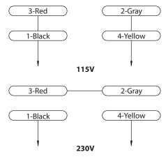
Figure 5 - Wiring Diagram
