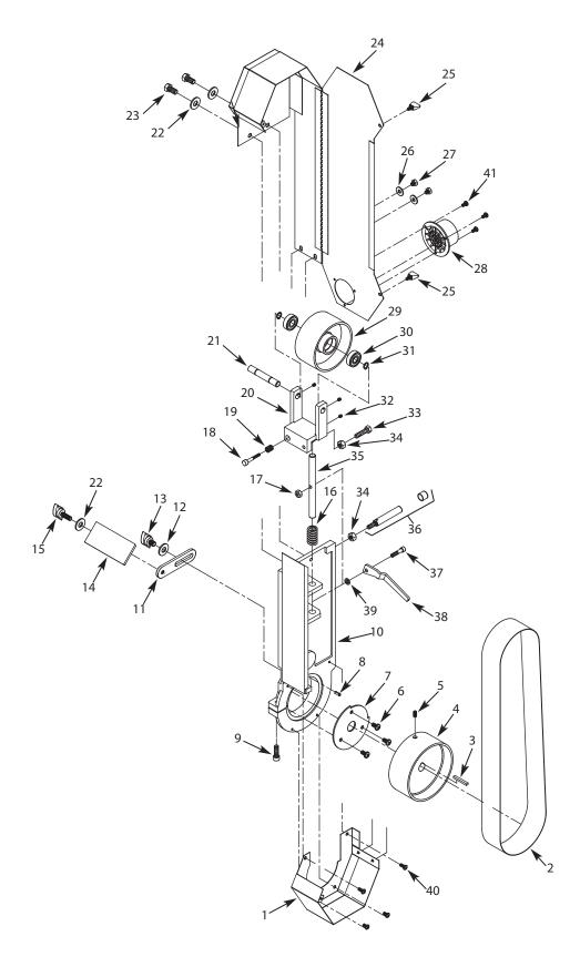
Figure 7 – Repair Parts Illustration for Housing
