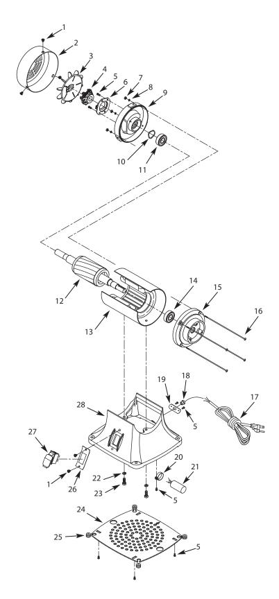
Figure 6 - Repair Parts Illustration for Motor
