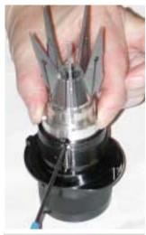
6. Remove wrench and reinsert into the set screw hole above the slot.
