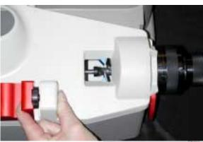
Drill point should be touching the end of the pusher shaft cap.
