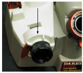
The first stage to sharpening a drill starts with the alignment process. In the alignment process, you will go through a few necessary steps prior to sharpening. Setting the material removal amount, adjusting the alignment tube to produce desired relief amount. Use athe Darex EZ align to set the drill to length and time the cutting edge.
