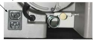
The power inlet is located at the bottom of the power receptacle.
