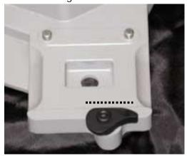
2. Position the sharpening fixture so that the 2 location holes on the base of the alignment fixture are aligned with the 3/8 dowel pins.
