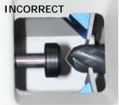
8. Once the drill has been aligned correctly and without releasing the slide handle, tighten the chuck knob clockwise until the chuck jaws grip the drill securely. Release the slide handle and remove chuck from alignment tube.
