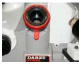
move the lever, it backs the chuck tube away from the wheel or moves it closer into it.
