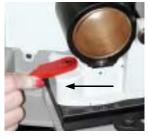
5. Before sharpening, make sure the sharpening fixture is secure and no longer slides in either direction.
