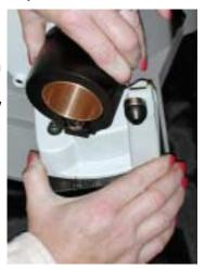
Insert the chuck with the thickest part of the cam touching the swing bearing.
