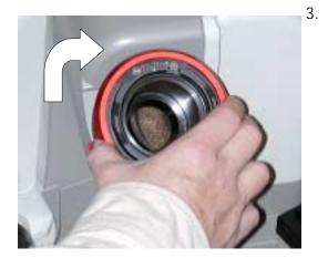
Rotate the adjuster counter clockwise to decrease the split angle.
