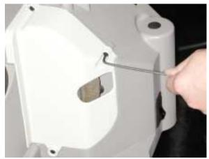
Using a 3mm hex key, remove 3; 3mm socket head cap screws (PP12240FF) from wheel guard cover.
