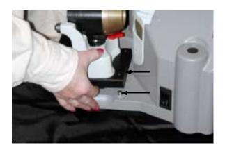
3. After sharpening fixture is in place, rotate the locking lever clockwise until snug. This will secure the fixture to the base.
