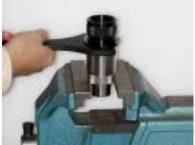
Rotate wrench clockwise to remove chuck knob/jaw assembly from chuck body.
