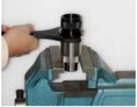
Rotate wrench counterclockwise to remove chuck knob/jaw assembly from chuck body.
