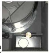
not let the tray become more than 1/3 full. To remove tray, unscrew brass thumb screw. Remove tray and dump contents. Wipe excess dust from the tray with a rag.
