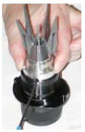
Remove wrench and reinsert into the set screw hole above the slot.
