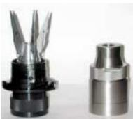
3. Using a 2.5 mm hex wrench remove set screw.
