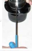
4. The internal pieces must remain keyed in order to remove the closing screw from the chuck knob assembly. Insert the 2.5 mm wrench into the set screw hole.
