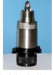
3. Holding the chuck in a horizontal position insert the drill into the appropriate sized chuck. (Sizes are on the cam).
