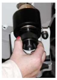
edges, avoid stopping when the drill is in the grind. Do not reposition your hand in mid-sharpening wait until the drill rotates off the wheel. Continue rotating the chuck in 360 degree rotations until the grinding noise is minimized to a near silence.
