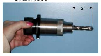
4. Rotate the chuck knob clockwise, which closes the chuck jaws onto the drill. Then slightly loosen the chuck jaws by rotating the chuck knob counterclockwise, about ½ turn. To determine how tightly the drill should be held during the alignment process, the drill should slide freely and drop out when the chuck is held in a vertical position.
