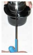
5. The internal pieces must remain keyed in order to remove the closing screw from the chuck knob assembly. Insert the 2.5 mm wrench, into the set screw hole.
