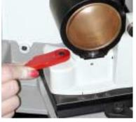
2. Place fingers on each side of the sharpening pivot base casting.
