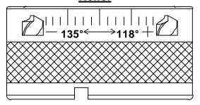
2. To increase or decrease the amount of heel relief produced during sharpening, change the position of the alignment tube.
