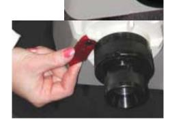
This will allow you to rotate the alignment tube in either direction.
