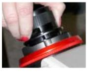
slots on the point split tube. Let the weight of the chuck ease the drill down and onto the grinding wheel. With slight pressure, be sure the chuck stays seated in the point splitter.
