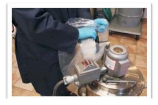
Place a poly liner around the now exposed HEPA/ULPA filter. Carefully remove the HEPA/ULPA filter from the back plate. Gently place the HEPA/ULPA filter into the poly liner. Gently twist the poly liner and then seal it with a tie wrap.
