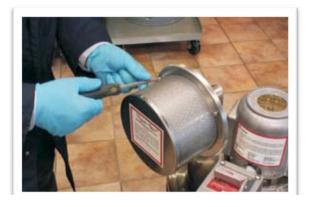
Remove the 3 screws on the HEPA/ULPA housing using a Philips Screw Driver.
